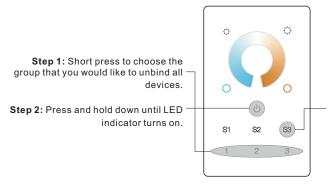
Step 3: Short press 5 times continuously to clear all bound lighting devices . LED indicator flashes 4 times for successful unbinding.
