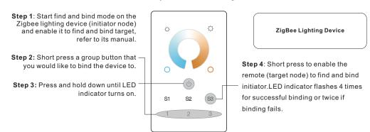
Note: Each remote can bind max. 30 lighting devices.
