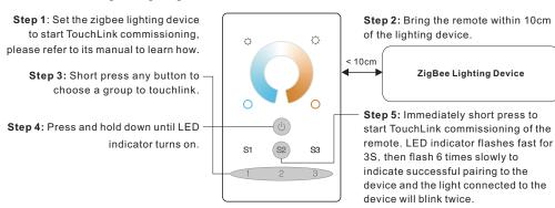
Note: 1) Directly TouchLink (both not added to a ZigBee network), each remote can link with 30 devices.
