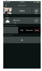
From your ZigBee controller or hub interface, choose to delete or reset the remote as instructed, indicator flashes 3 times quickly to indicate successful removing.
